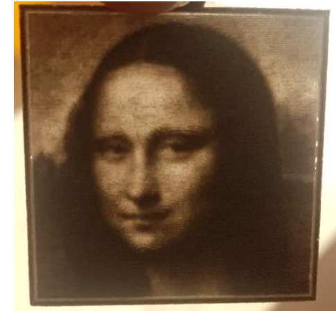
MJF part printed at 45° with a minimum thickness of 0.08mm
